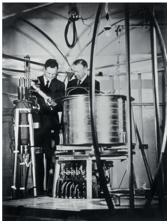
Fig. 1. Manne and Kai Siegbahn together at the first ESCA spectrometer, mid 1950s
